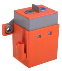
The new EVC 250 features larger contact gaps, optimized switching dynamics, high performance arc suppressing magnets and other measures to effectively control the switching arc. The contactor achieves continuous current ratings of 250A which ensures a safe short circuit carry capability of 6kA and complies with the demanding switching requirements in hybrid and electric vehicles. Service replacement due to pressure loss or gas leaking is no longer necessary.
