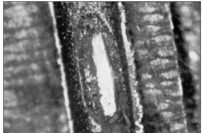
Figure 2: The polished section of a plated-thru hole shows a clean contact area. The remaining plated-thru area has visibly changed due to industry atmosphere.
