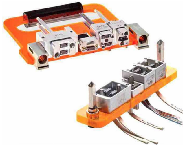
IMAGE: TE Connectivity's ruggedized optical backplane interconnect system meets VITA 66.1 and 66.4 open architecture specifications for VPX systems and provides a high-density, blind-mate optical interconnect in a backplane/daughtercard configuration. The fiber optic ribbon cable interconnect feeds through the backplane to removable system modules using MT ferrules.
