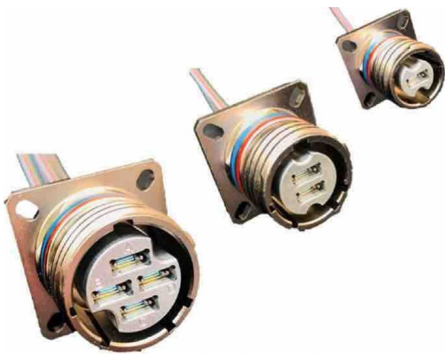
IMAGE: TE Connectivity D38999 Series III Style Circular Connectors with a self-locking, anti-vibration coupling mechanism and up to four MT ferrules capable of accommodating up to 96 optical channels.
